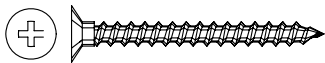
2 EACH - 1 1/4" LONG PHILLIPS FLAT HEAD SCREWS FOR ATTACHING LIGHT RAIL - ACTUAL SIZE SHOWN
