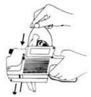
4. Feed labels through labeler allowing an extra 4 inches to extend below base plate.
