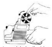
2. Insert label roll with tape going over top of guide. Close compartment.
