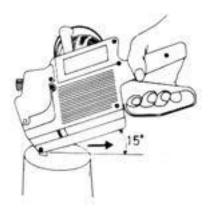
To affix label, squeeze handle and touch onto merchandise with a rolling motion, lifting handle approx. 15°.
