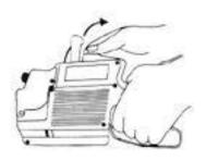
1. Pull out tab and lift the label compartment in the direction of arrow.
