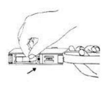
5. Close base plate and remove labels from backing. Insert end of label tape into slot marked "LABEL" (behind base plate, not the small narrow slot.)
