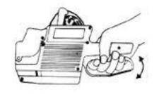
6. Squeeze handle 7-8 times to feed tape around pin-feed wheel and out the back slot.
